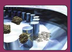
After impacting against the rotor pins, feed material is discharged off the rotor against a stationary liner for further particle size reduction.
