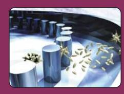
After impacting against the rotor pins, material is discharged against the stationary liner for further deagglomerating.
