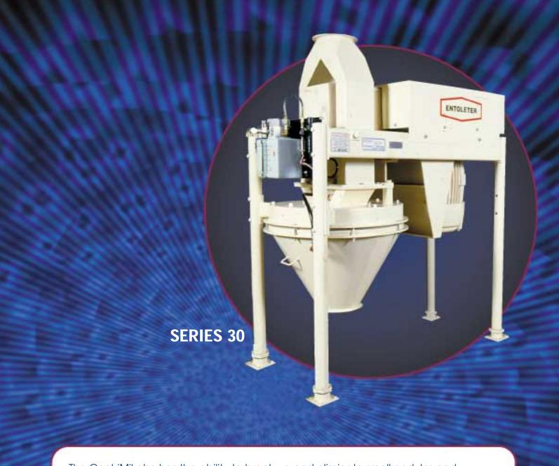
The CentriMil also has the ability to break up and eliminate small nodules and agglomerates which may form during the mixing process. This is of particular importance in such industries as pharmaceuticals, plastics, and coatings.
