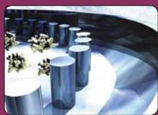
Agglomerated material enters through the top of the CentriMil and is distributed onto the spinning rotor. Centrifugal force hurls the material outward at high speed.
