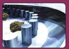
Feed material enters through the top of the mill and is distributed onto the spinning rotor. Centrifugal force hurls the material outward at high speed.
